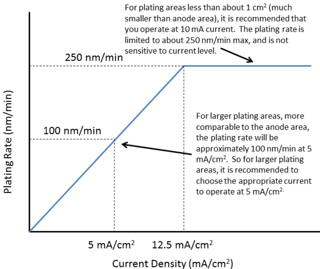
**2.5.11** Set up the power supply. You want to operate in constant current mode (current limited mode) to get a constant deposition rate. In order to accomplish this:
