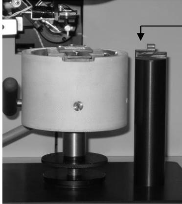
This height should be ~4.27" above the large black baseplate ... the height you are bonding at.
