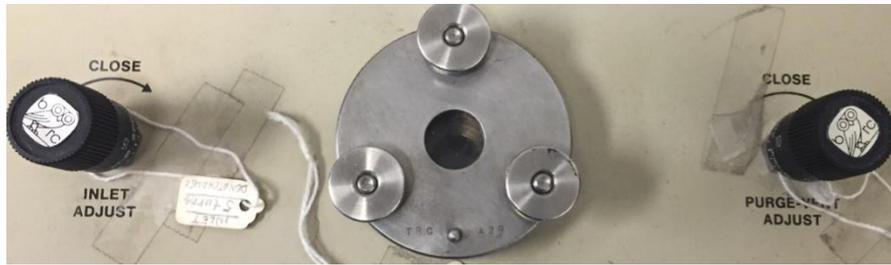
**Figure 1 - Front panel of Critical Point Dryer (CPD)**
