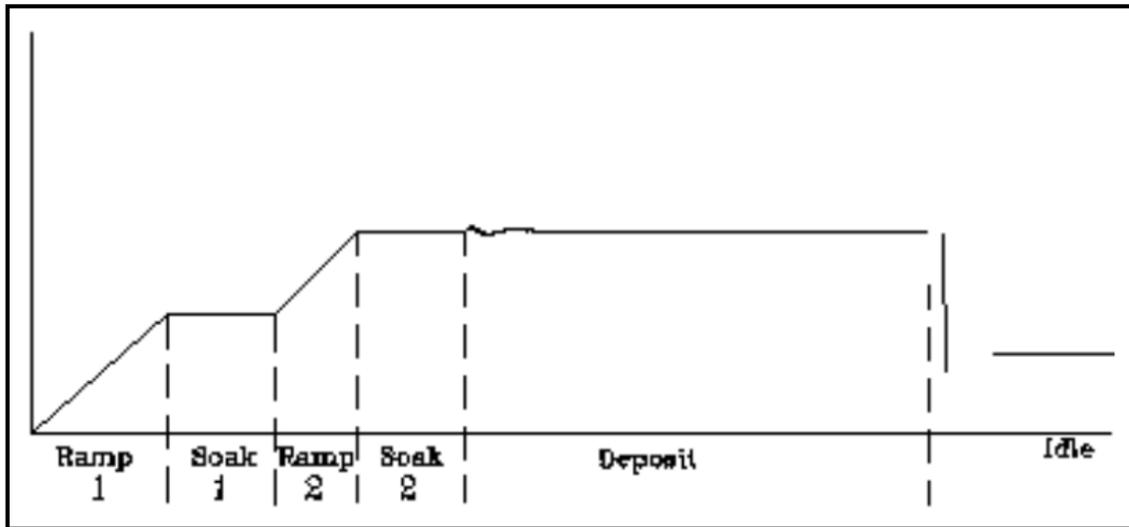
16. Once your desired thickness is reached, the system should automatically close the substrate shutter and ramp the power back down to zero..
